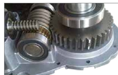
Bronze and tempered steel internal gears for maximum reliability
